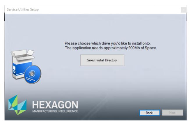
Click on Select Install Directory to select the drive which you would like to install the Service Utilities on. (This is the initial drive and path not the final name of the Service Utilities Directory)
